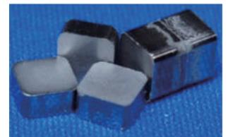
▲High heat-resistant Sm-Fe-N anisotropic sintered magnet
